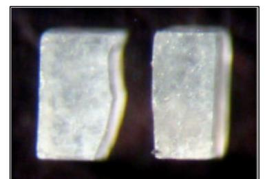
**Left** is cut specimen from clay. **Right** is cut specimen from thermal wax
